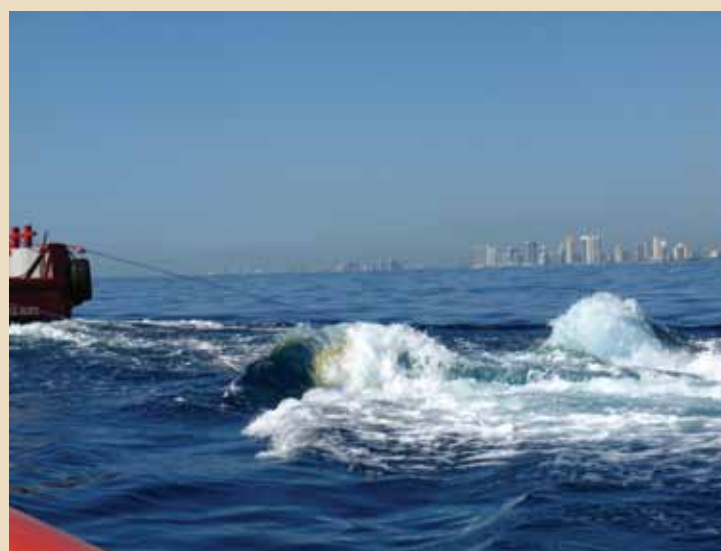
Figure 4 Photo of a wake created by chute with short trailing distance
