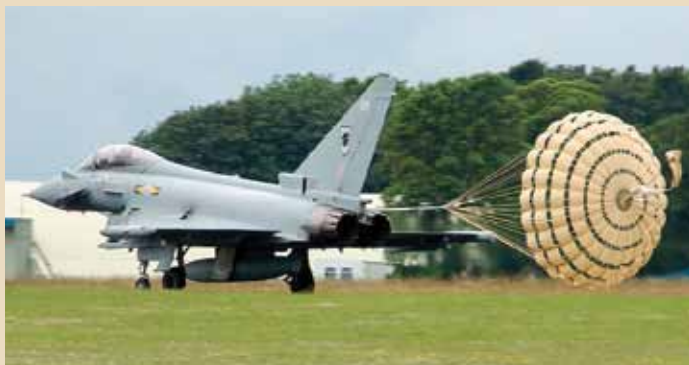
Figure 1 Illustration of the concept on the typical usage of drogue chutes deployed astern of fighter jets versus the proposed usage of drogue chutes for large ships
