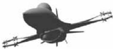
Figure 3 Wing deformations due to aircraft manoeuvre loads on wing
