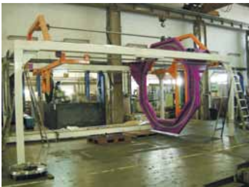
Figure 3 Partial assembly of a multi-axis braiding machine
