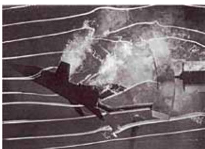
Figure 5 Flow separation of an aircraft at a high angle of attack
