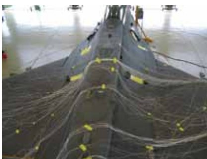
Figure 6 Ground vibration test set-up
