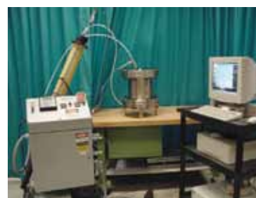
Closed-mould RTM process
