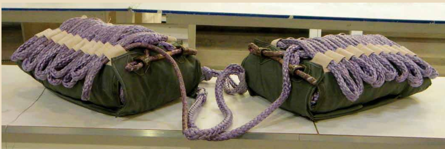
Figure 5 Packed Deployable 1/8 th Scale System with two ribbon chutes in each bag
