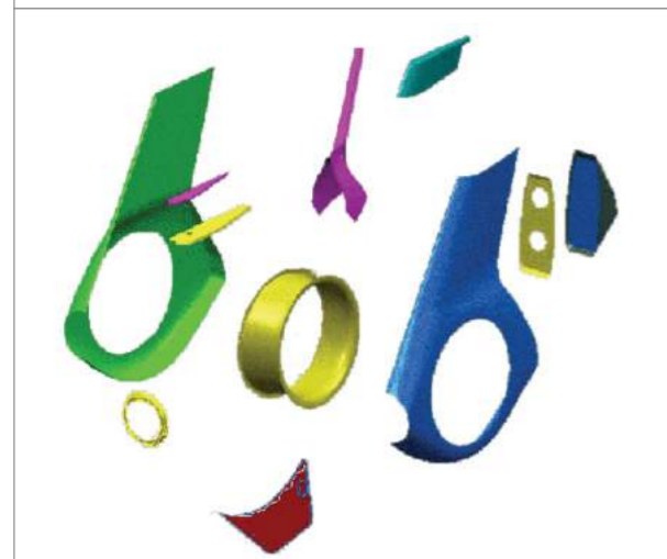
EC-120 rear structure
