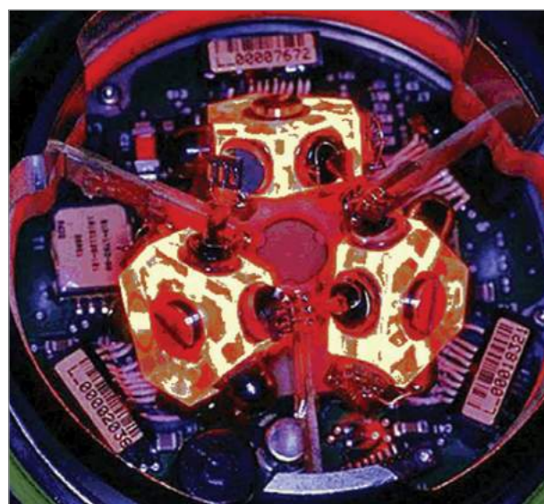
Three identical Ring Laser Gyroscopes arranged in Orthogonal axes
