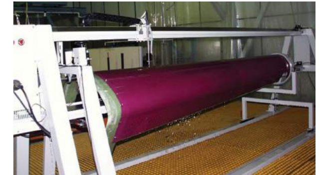
Ultrasonic scanning to check for defects
