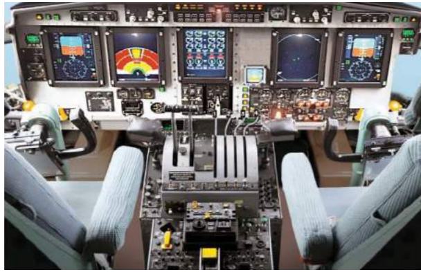
The upgraded RSAF C-130 with a modern glass cockpit, with the EIDS located at the centre of the five glass displays
