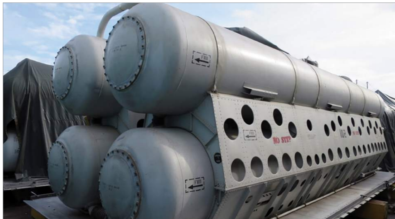
Internal fuselage mounted fuel tanks for KC-130
