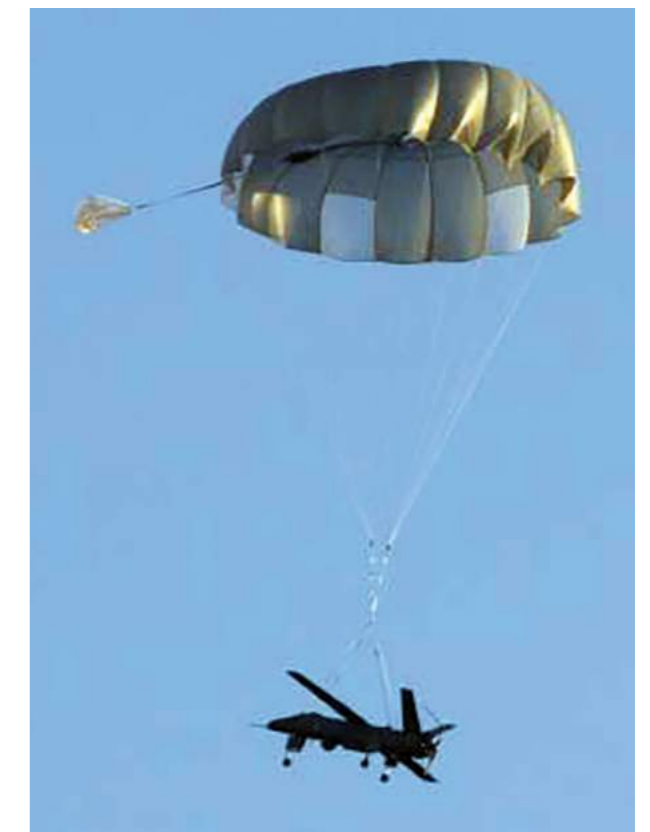
Parachute recovery for Skyblade IV
