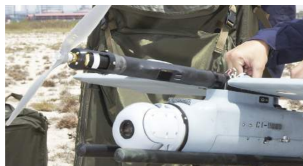
Modular payload on Skyblade III
