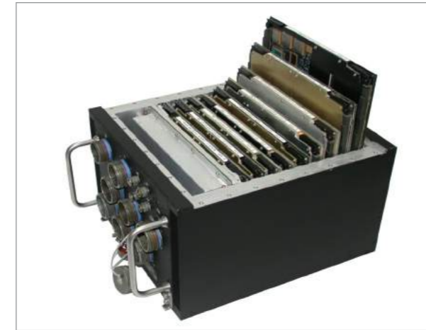
Mission computer used in SP Avionics upgrade with top cover removed, showing shop replaceable units
