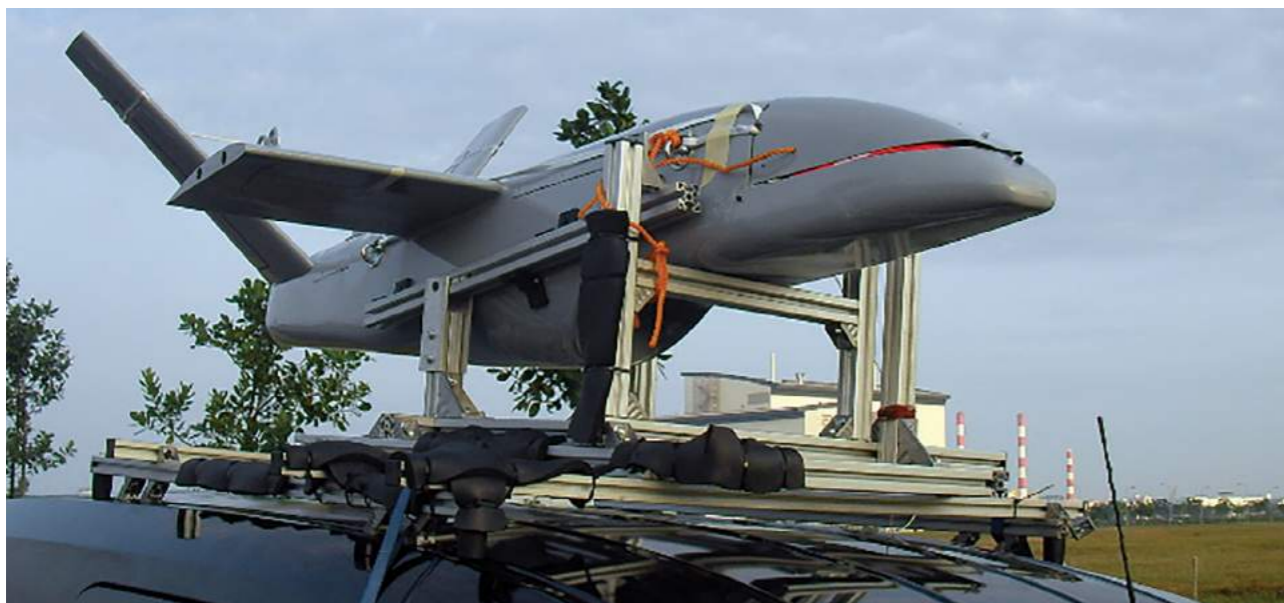
Skyblade IV mounted on top of a vehicle in ground test
