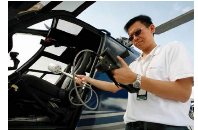
Electromagnetic-field measurements of an EC-120 trainer helicopter
