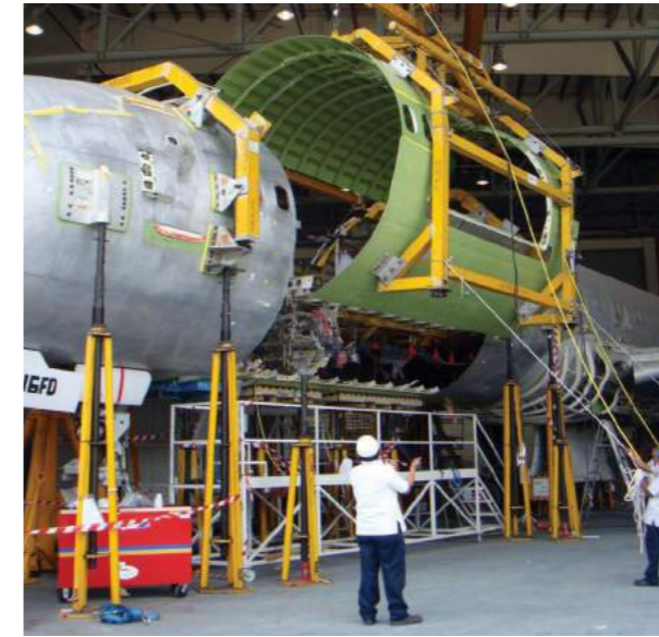
B757 conversions undertaken at STA Engineering, Singapore
