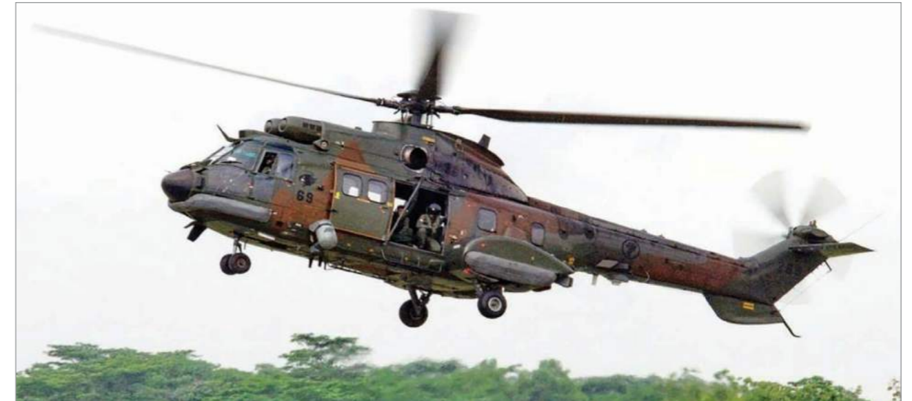
Upgraded Super Puma with FLIR turret deployed
