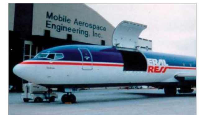
First converted B727 freighter carried out by MAE
