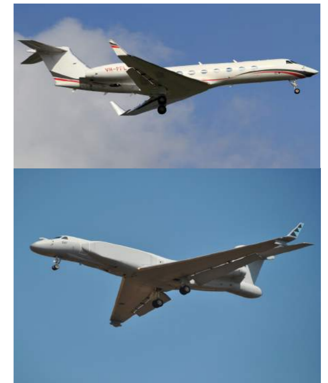
G550 before and after modification with airborne sensor
