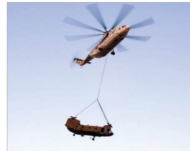
A chartered civilian MI-26 lifting a damaged MH-47E Chinook at an altitude of 2600m in the mountains near Sirkhankel, Afghanistan
