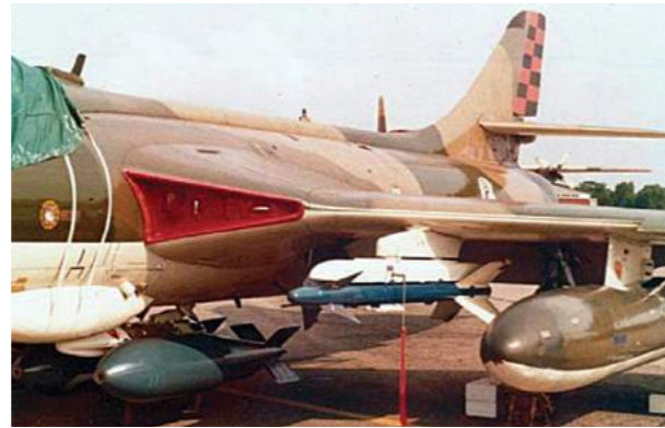
The only Hunter aircraft to have AIM-9 missiles and centreline MERS carriers
