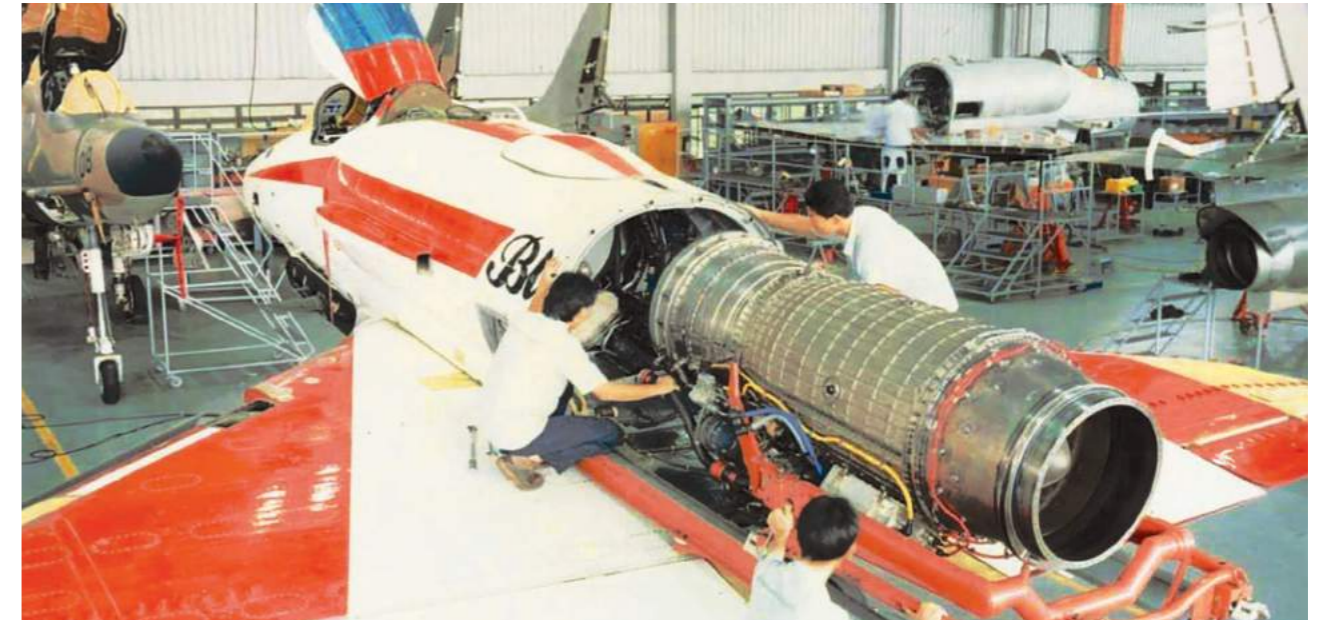
A-4 in Black Knight colours with rear fuselage split for F-404 engine removal
