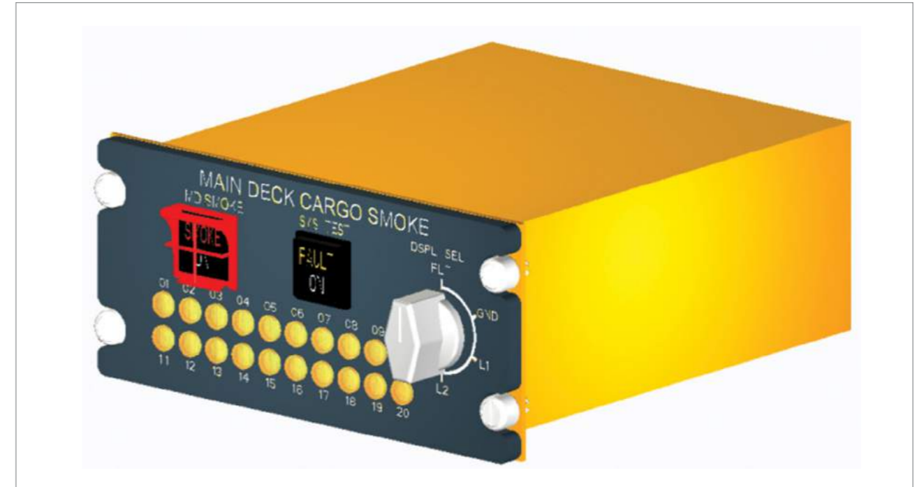
Computer-aided design image of main deck cargo smoke control panel for the A330 freighter
