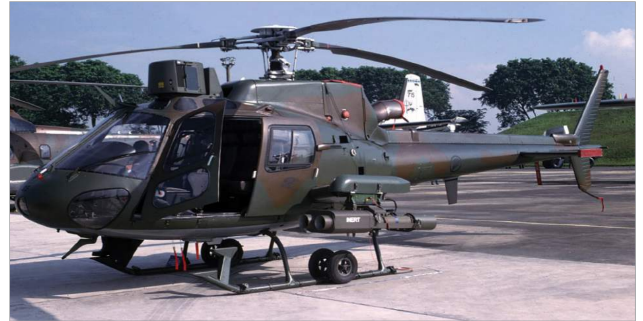
Fennec fitted with TOW missile and gun pod
