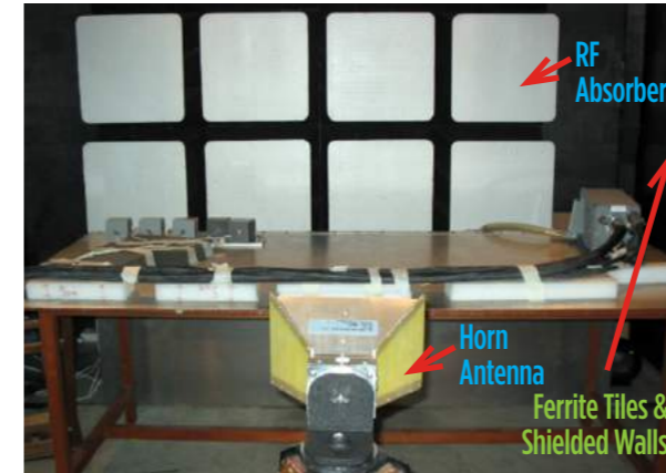
Product EMC testing in a semi-anechoic chamber
