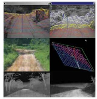
Results from the passive perception systems: stereovision (top two), colour segmentation (middle left), slope analysis (middle right), and infrared images (bottom two)
