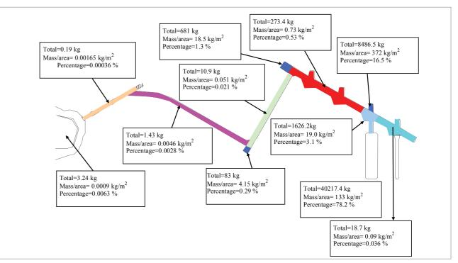
Large scale test results from case charge test showing the distribution of debris mass inside the tunnel and the effectiveness of debris traps in reducing debris hazards
