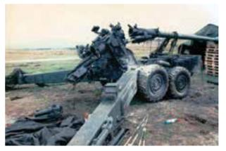
Damaged FH2000 Gun from an in-bore explosion
