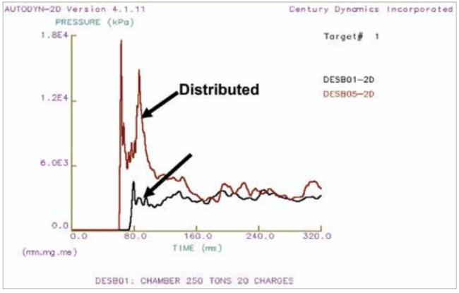
Significantly lower chamber blast pressure on blast doors from distributed charges compared to a single charge of the same mass, resulting in significant savings in blast door design.
