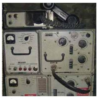
AN/GRC 103 multi-channel radio relay system
