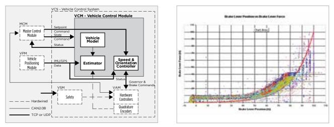
Vehicle controller configuration (left) and the non-linearity when one of the control levers was used to steer the vehicle
