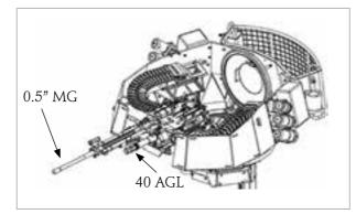
Cupola platform with twin weapons concept (40mm automatic grenade launcher and 0.5" machine gun) for M113
