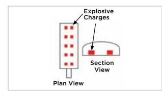
Setup for explosives with distributed charges to simulate realistic storage conditions
