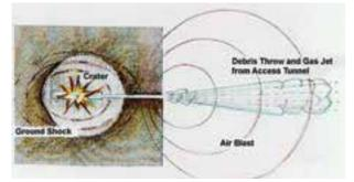
Illustration of the effects of underground explosion (plan view)
