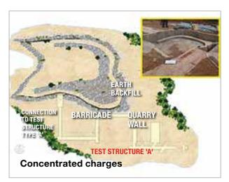
Layout for small-scale tests including key features of the tunnel system and external barricade and quarry walls
