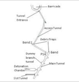
Layout of the test facility based on a simplified storage cluster with the key tunnel and safety features
