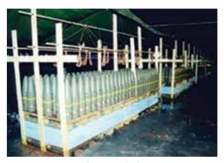
Setup for cased charges with 155mm artillery rounds to represent the worst case scenario for debris hazards
