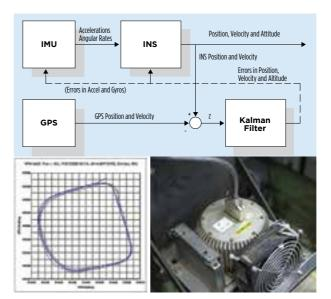
The localisation system configuration (top) used and the results obtained (bottom left) on a vehicle that by its nature will vibrate very much during motion
