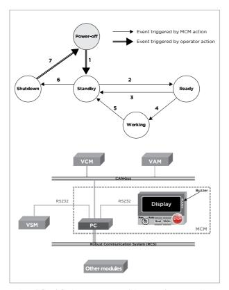
Simplified finite state machine and supervisor hardware configuration
