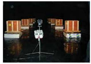
Setup for the bare charge tests to serve as the reference for comparison of explosion effects in air blast, ground shock and debris hazards
