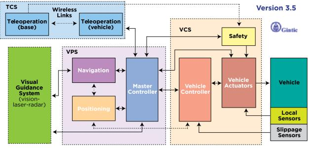
Ulysses vehicle System Block diagram
