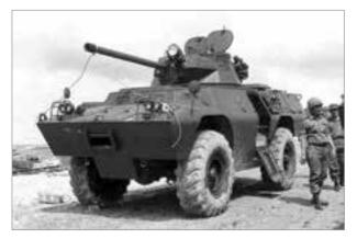
90mm gun on the V-200 with rope to limit angle of traverse for live firing at Sungei Gedong live firing range, circa 1970
