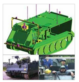
Clockwise from top left: M113 CAD model including sensor details, the APC with the sensors outfitted and demonstration with the driver's hands outside the vehicle to prove that the vehicle was moving autonomously.
