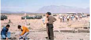
Explosion with 4176kg of Tritonal destroyed the shelter completely as the door of the shelter had prevented venting of the blast
