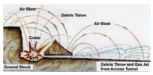
Illustration of the effects of an underground explosion (section view)
