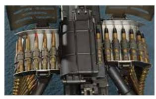
Left & Right Feed of CIS50MG, with feed covers open
