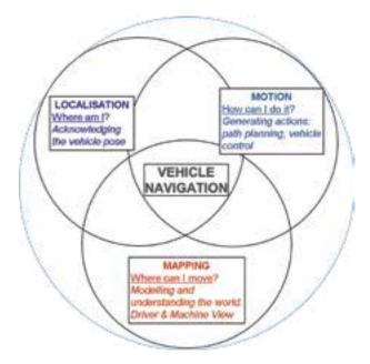
Functions addressed by Ulysses for autonomous vehicle navigation
