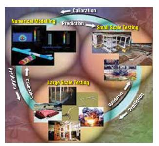
Systematic approach to technology development following a feedback loop for numerical modelling, small-scale testing and large-scale testing
