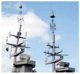
The pre-upgrade MCV with its slanted mast (left) compared to the upgraded MCV with its straight mast (right).
