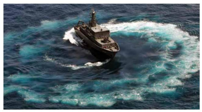
An MCMV demonstrating the sort of maneuverability provided by its Voith-Schneider propellers.
