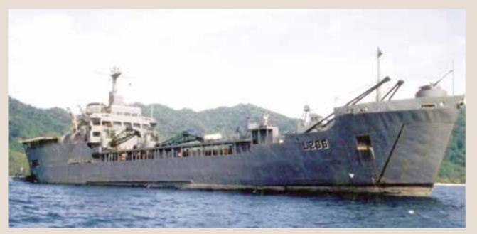
One of the old County-class landing ship tanks, designed for amphibious operations and landing troops and vehicles directly onto a shore.
