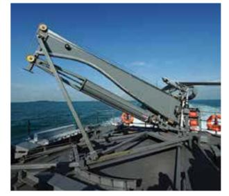
The design of the modified UAV launcher installed aboard the corvettes after the upgrade added additional functionality through a turntable.
