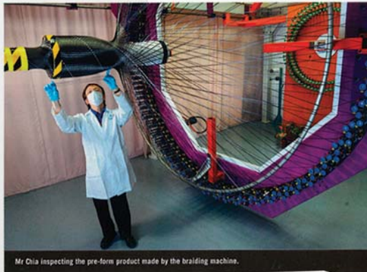
Mr Chia inspecting the pre-form product made by the braiding machine.
