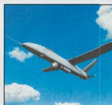
The locally made Skyblade IV can travel up to 100km and can be airborne for up to 12 hours. Final technical flight tests are being run before army troops test it at the end of the year.
