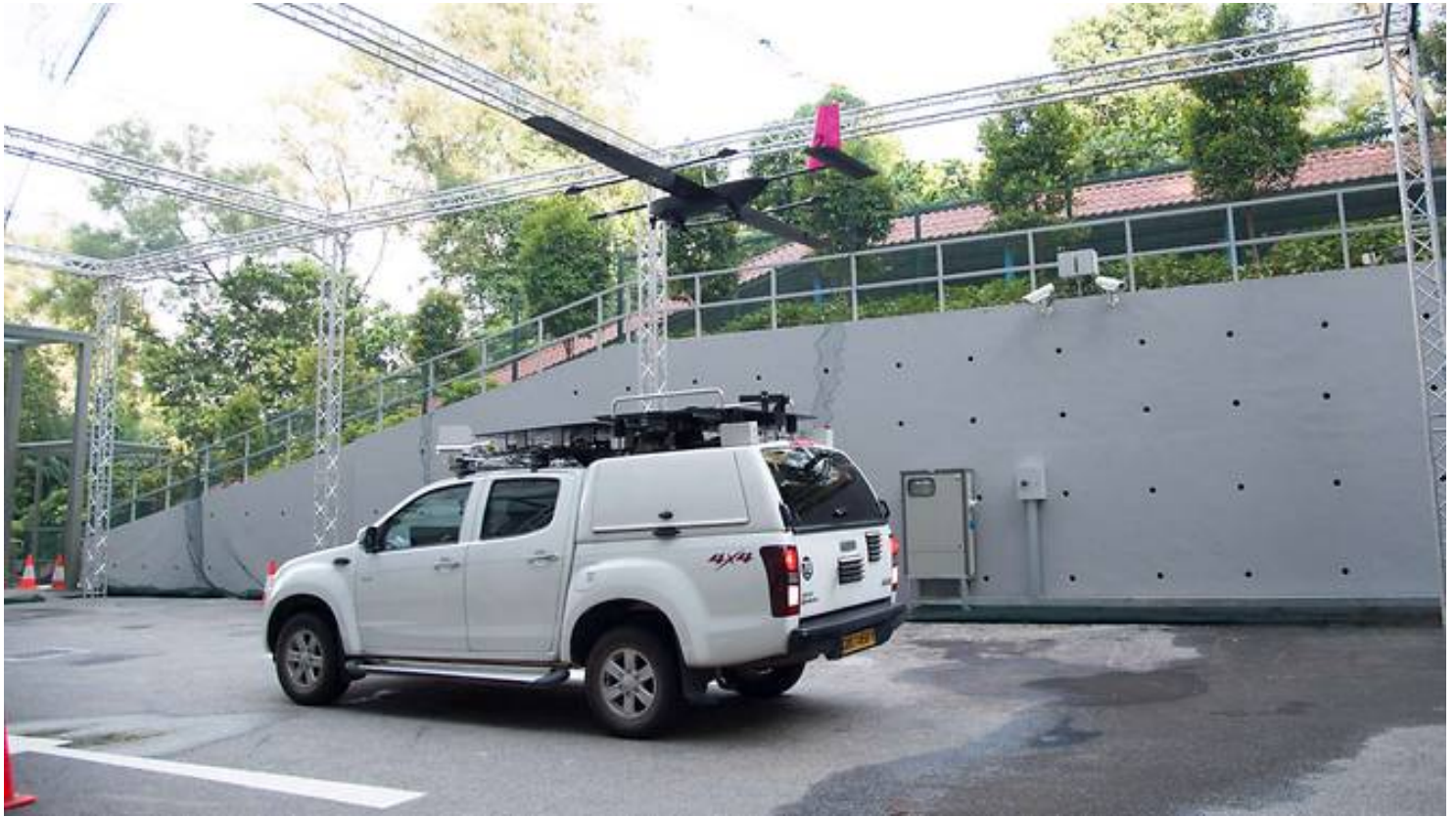
The unmanned ground vehicle can navigate without GPS by using lasers or cameras. (Photo: DSO)
