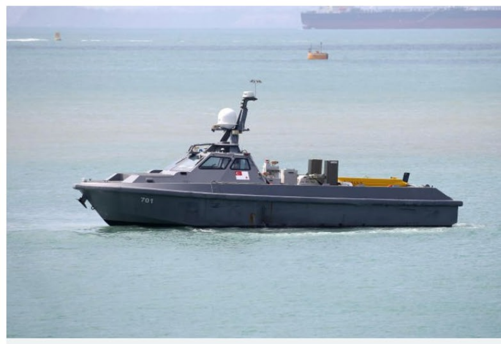
The unmanned surface vessel (USV) takes about six minutes to deploy sonar equipment, with two operators controlling the ship remotely. ST PHOTO: SEAH KWANG PENG
