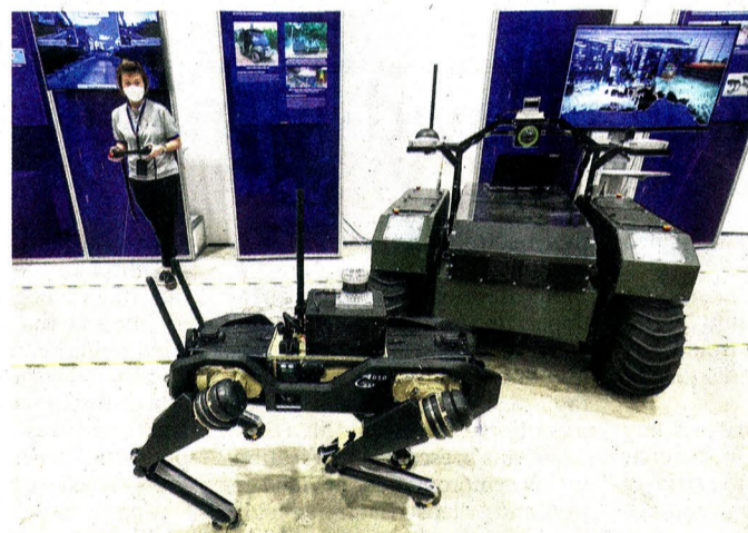
Harrier (front), a robot that can be used for surveillance in urban areas, at DSO National Laboratories' 50th anniversary exhibition. ST PHOTO: GAVIN FOO
