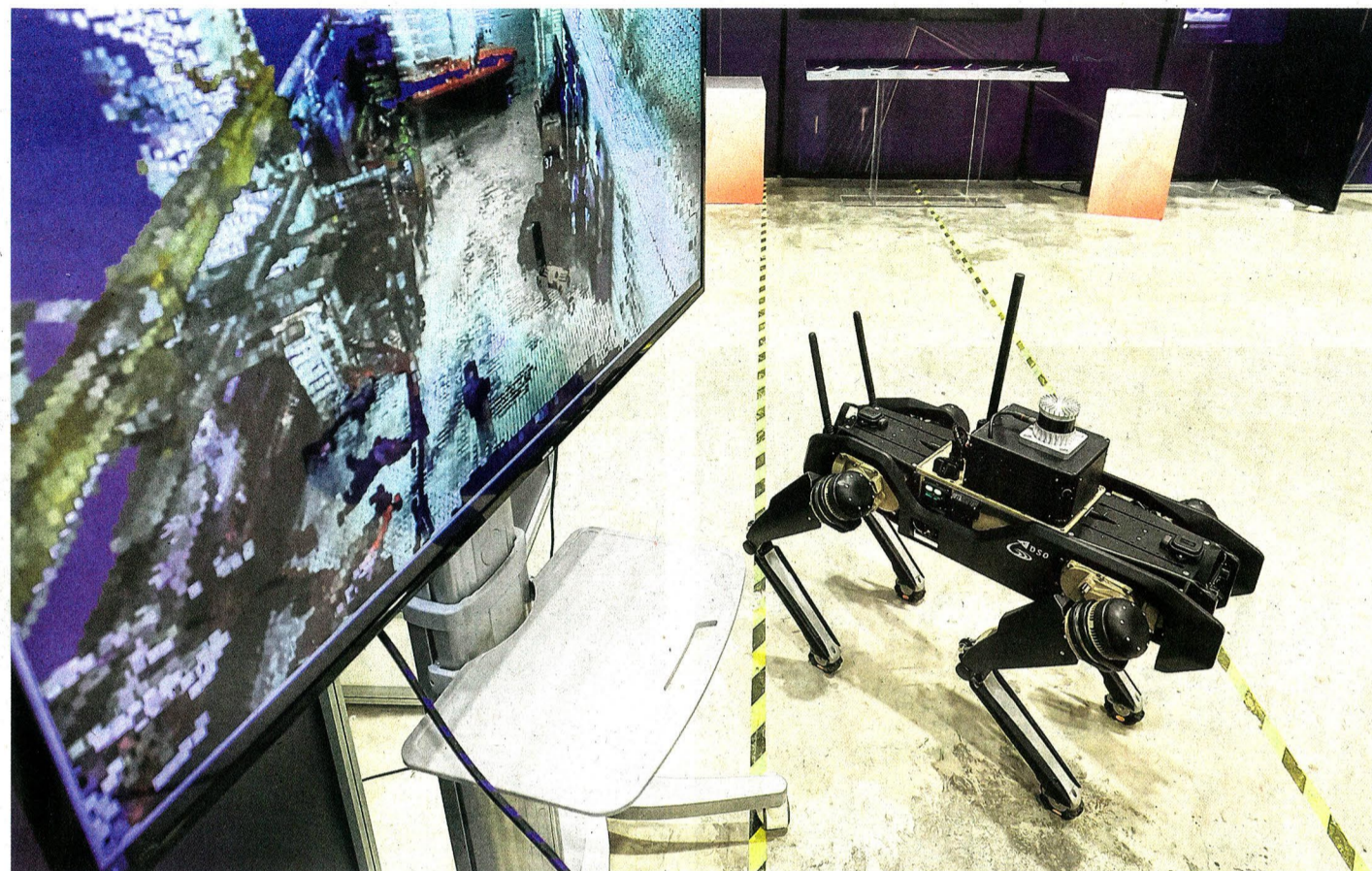
Harrier, a robot that can manoeuvre through tight spaces and narrow corridors, and even climb stairs, on show at DSO National Laboratories' 50th anniversary exhibition at the DSO Complex near Kent Ridge. The robot will be used to conduct surveillance in urban environments. ST PHOTOS: GAVIN FOO
