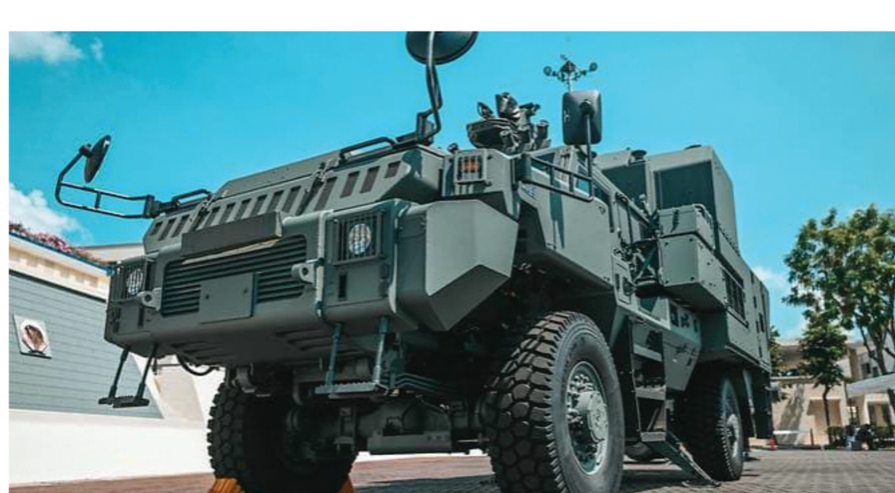
The BELREX Protected Combat Support Vehicle (Mortar) is equipped with the 120mm Advanced Mortar System, requires less manpower and can be quickly deployed for responsive fire support. (Photo: Hanidah Amin)
