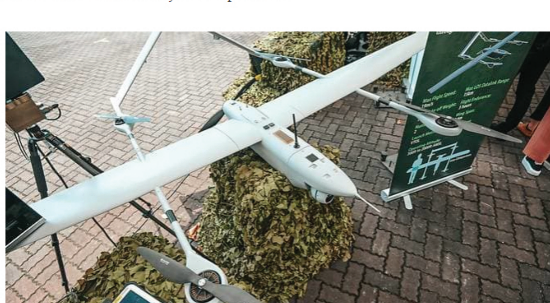
The VELOCE 15 mini-Unmanned Aerial Vehicle (V15 mUAV) has an improved operating range and can provide high-resolution live imagery to forces for real-time situational awareness. (Photo: Hanidah Amin)
