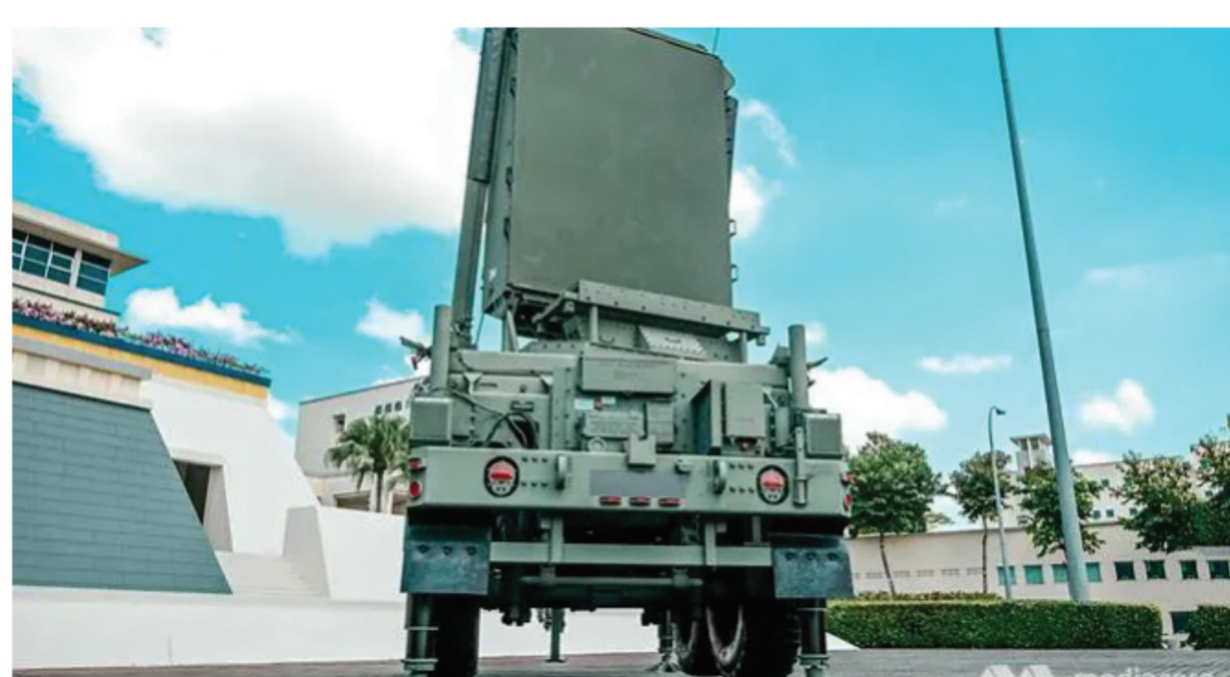
The TPQ-53 Weapon Locating Radar (WLR) is highly automated and requires about 30% less manpower to operate. (Photo: Hanidah Amin)
