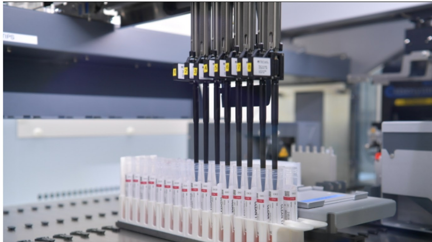
Automated pipettes are used during the preparation of samples for testing, to reduce testers' exposure to the virus.
