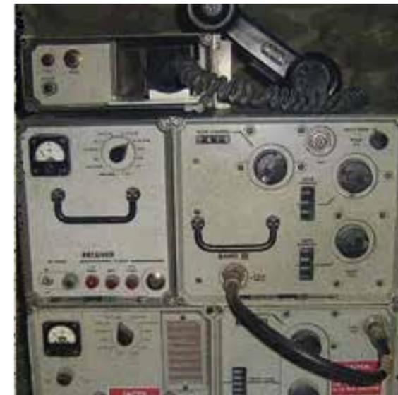
AN/GRC 103 multi-channel radio relay system
