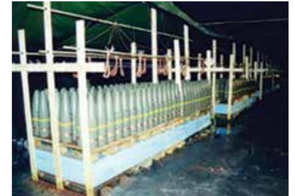
Setup for cased charges with 155mm artillery rounds to represent the worst case scenario for debris hazards
