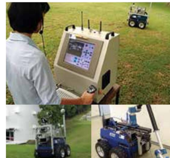
Different configurations of the platform used for tele-operation experiments
