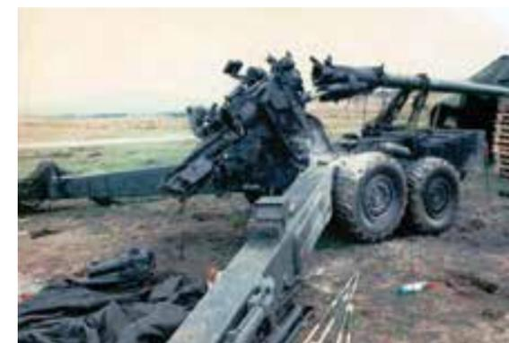
Damaged FH2000 Gun from an in-bore explosion
